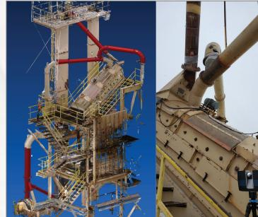
3D Scanned and Reverse Engineered Chute Systems
